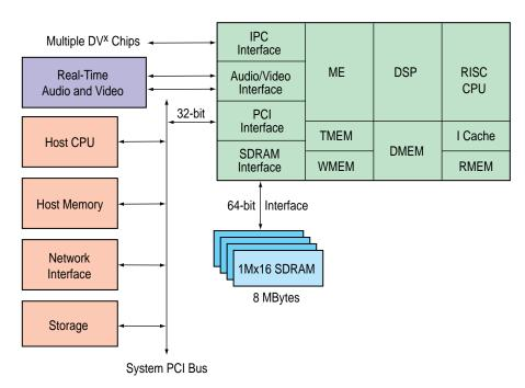
DV<sup>x</sup> Platform Architecture Block Diagram
